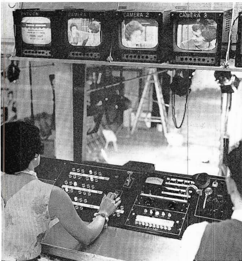
FIG. 9. The control panels for TS-40 switcher and special effects system are shown in the Studio B control room. The panel above the special effects selector includes camera intercom and studio talkback facilities for the technical director.
