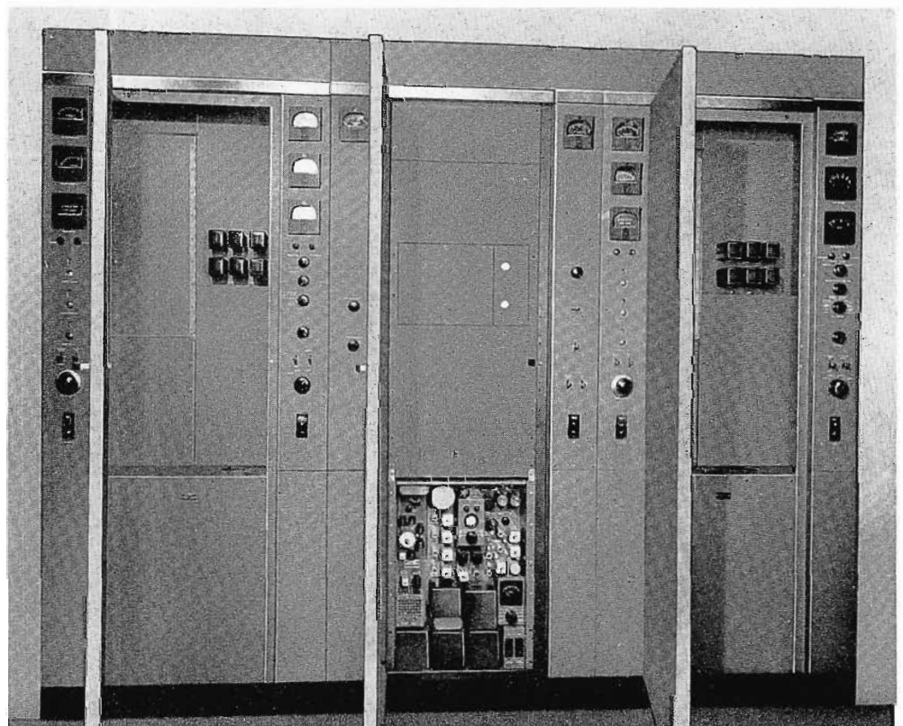
FIG. 2. Two identical 10-kw amplifiers are housed in cabinets at either end of the transmitter. Center cabinet contains "Direct FM" exciter and 400-watt driver.
