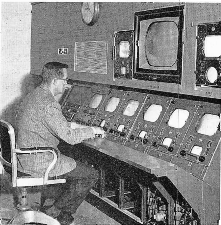
FIG. 18. Position for shading of film cameras in the master control area.
