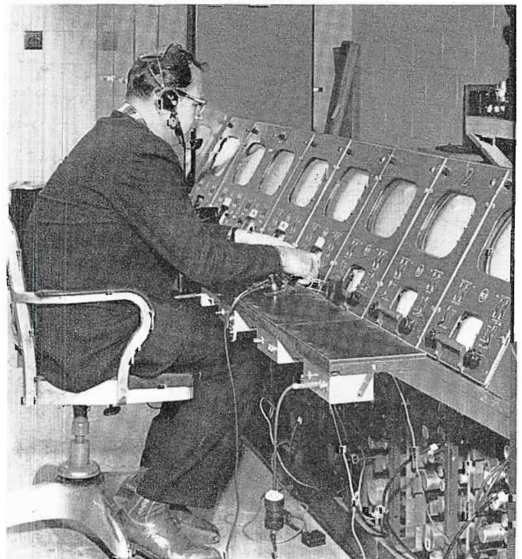
FIG. 19. Eight TK-11 cameras are adjusted from this position in master control.
