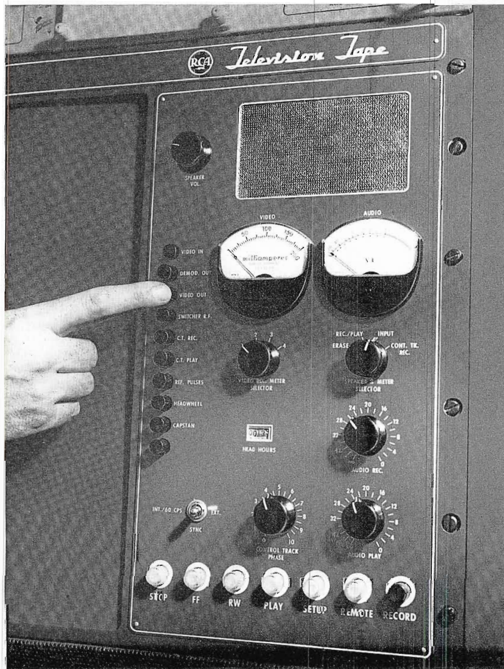
FIG. 6. Basic tape control functions are accommodated on this simplified control panel which also includes a monitoring switcher. In the panel adjacent to the control panel, space is available for mounting an accessory TM-35 Master Monitor which includes both picture and waveform presentations.
