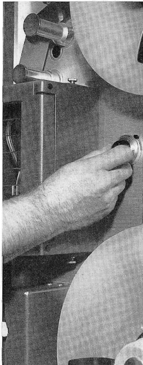
FIG. 7. This manual control mounted on the tape transport panel determines mechanical positioning of the vacuum guide. Thus, the operator can manually compensate for variations in head-to-tape pressure.
