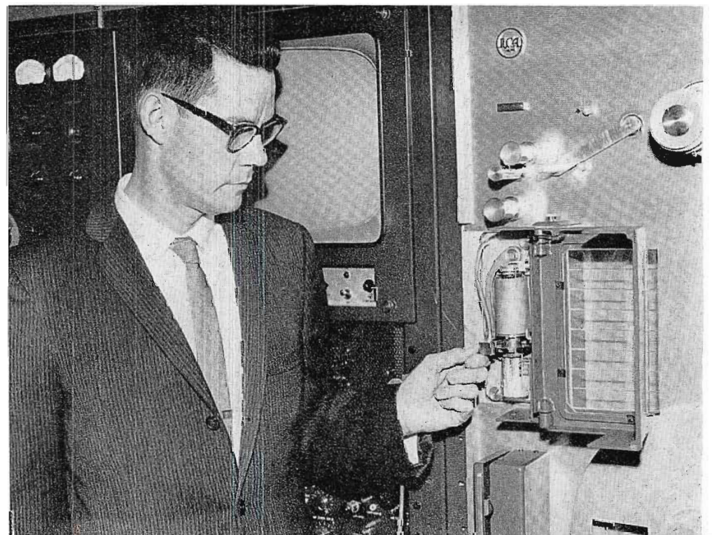
FIG. 1. The author, Frank Bateman, inspects one of the tv tape headwheel panels. In 5,000 hours of operation, WBTV has averaged 238 hours per panel, including those still in service. Seven separate headwheel panels have racked up over 300 hours each.
