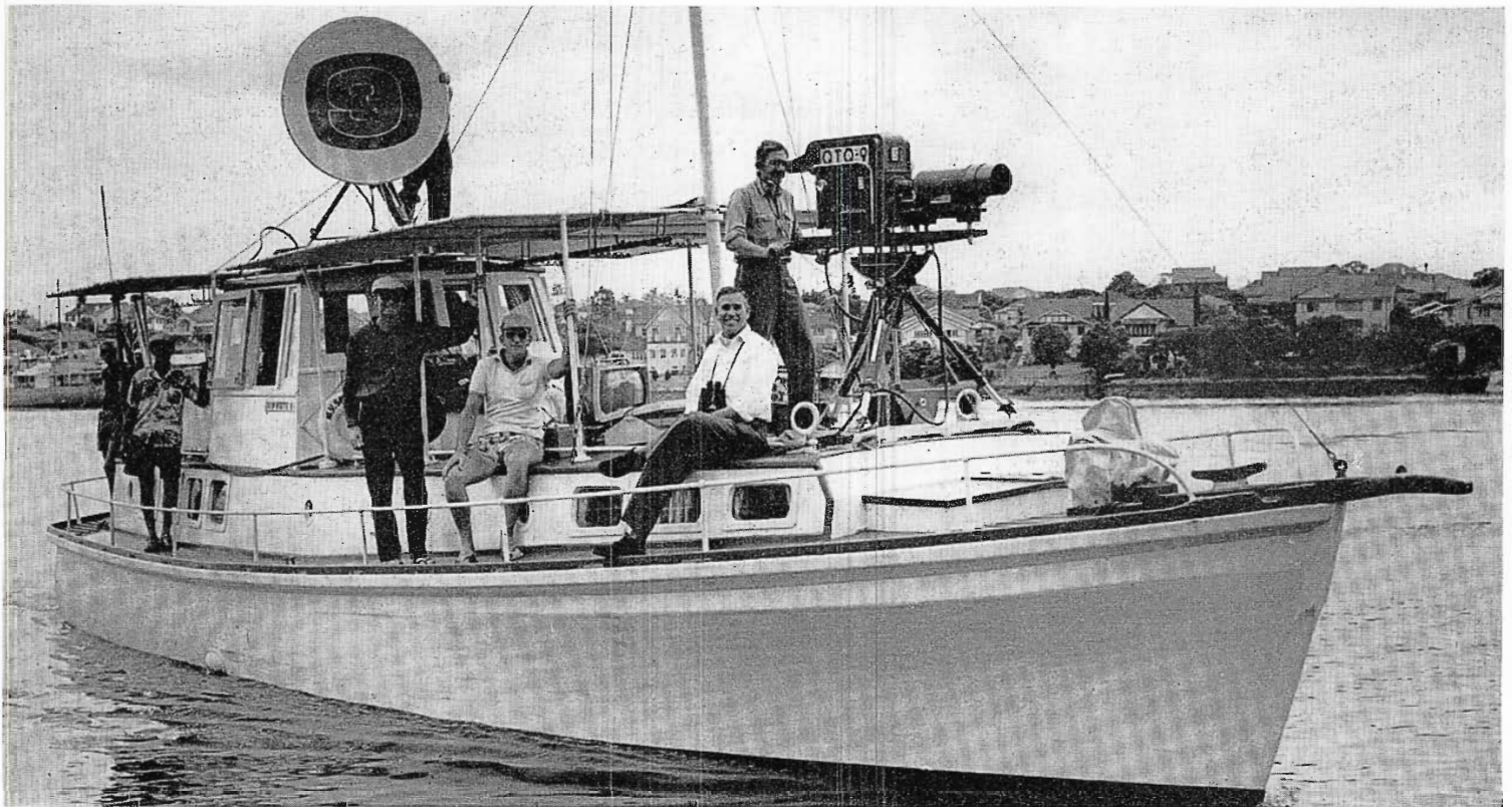
FIG. 16. A TVM-1A microwave link with 4-foot reflector and TK-31B Image Orthicon camera with zoom lens are seen mounted on a launch during a remote telecast of the 18-Footer Sailing Championships on the Brisbane River.
